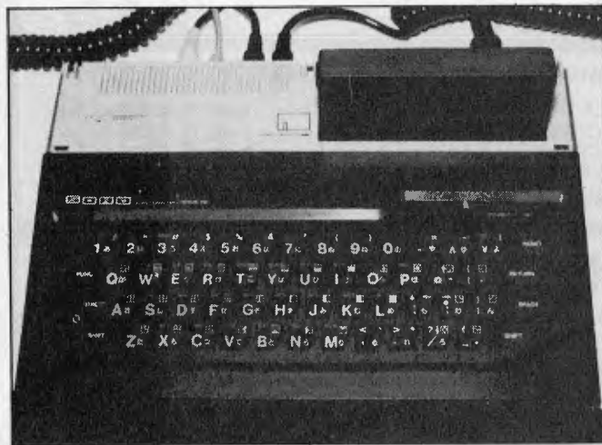
Sord's neat little home micro, the M5. Note plug-in ROM pack (16k).
